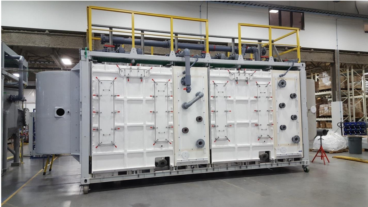
Figure 3 Effect Module: Built for modular dispatch to minimize site work
